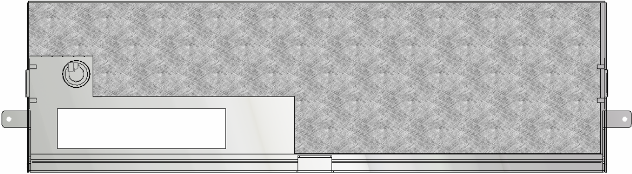
Figure 6-15 Align Dust Filter with Cut Out in Bezel
