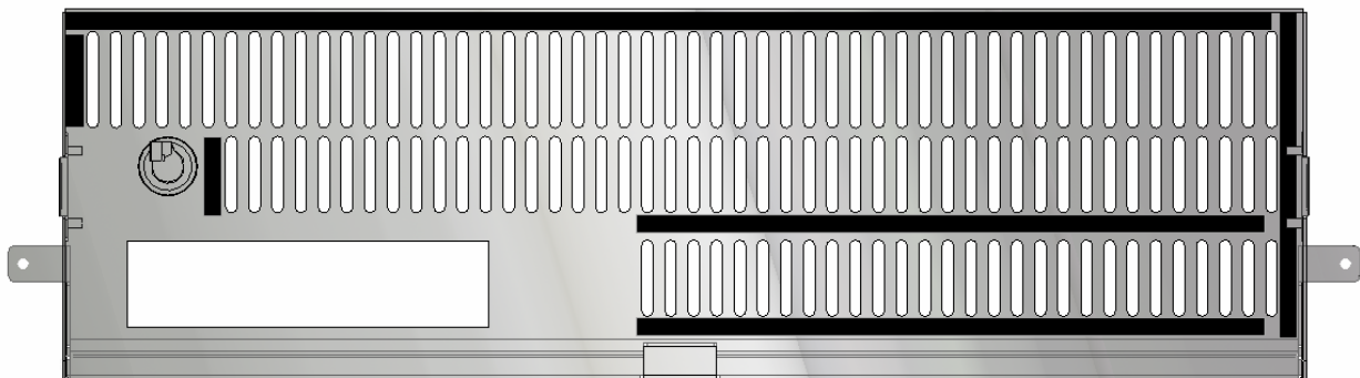
Figure 6-14 Location of Velcro Tape on Inside of Bezel
